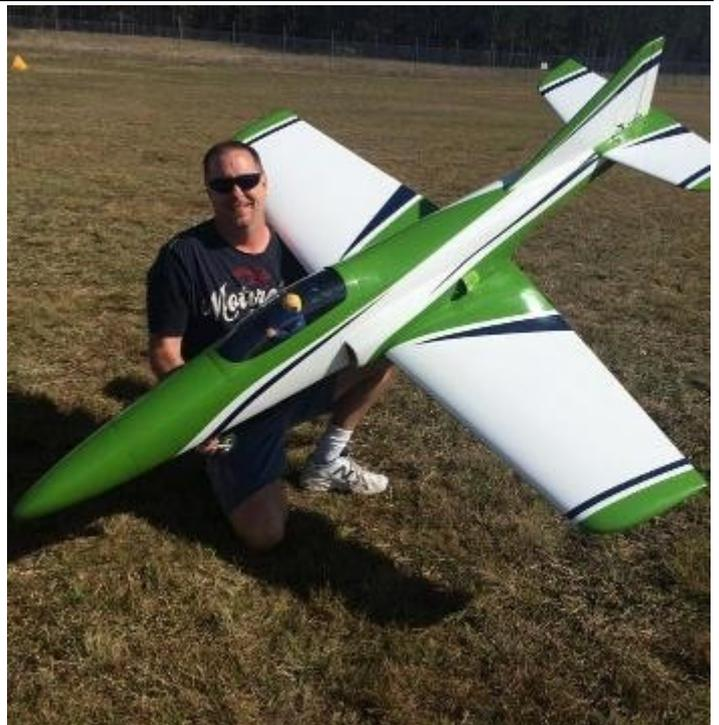
Fuselage is 2.2m long, wingspan 2m. All up weight including fuel and smoke fuel, 17kg. Engine is a Kingtech k140g kero start, 3.5L fuel tank for a 10 minute flight.
