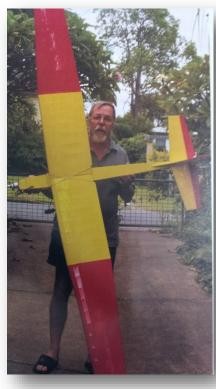
Back to Dave: I installed a Turnigy 3536/1100 motor and their 40amp ESC. These run on a 10 x 5 APC-'E' prop and the power comes from a 3S 3000 MAh Lipo pack. You may see from the photos that I built a ply box on to the fire wall to get the prop into the same location as the prop shown in the plan as it is designed for a .20 glow or similar. Other than that I built it pretty much as per kit. The fuselage is really strong with light ply sides.
