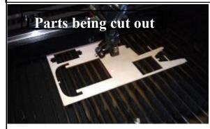
Bob's new Laser machine is now up and running. On his website (www.wolfmodels.net) he'll be listing the plans that he has in stock waiting for cutting short kits. The size he can cut is 2200mm long x 1200mm wide. So if you need a long fuselage side cut in one piece he can do it with ease. Send him your plan, either paper
